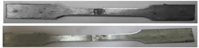
FIGURE 7: VaFSW TENSILE SPECIMENS BEFORE AND AFTER THE FRACTURE
