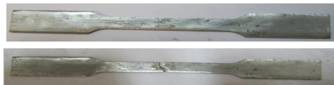
FIGURE 6: FSW TENSILE SPECIMENS BEFORE AND AFTER THE FRACTURE
